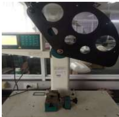
Figure 2. Tinius Olsen impact testing machine for measuring sample unnotched impact resistance.
