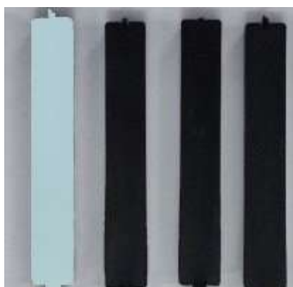
Figure 3. Sample used to measure unnotched impact toughness.
