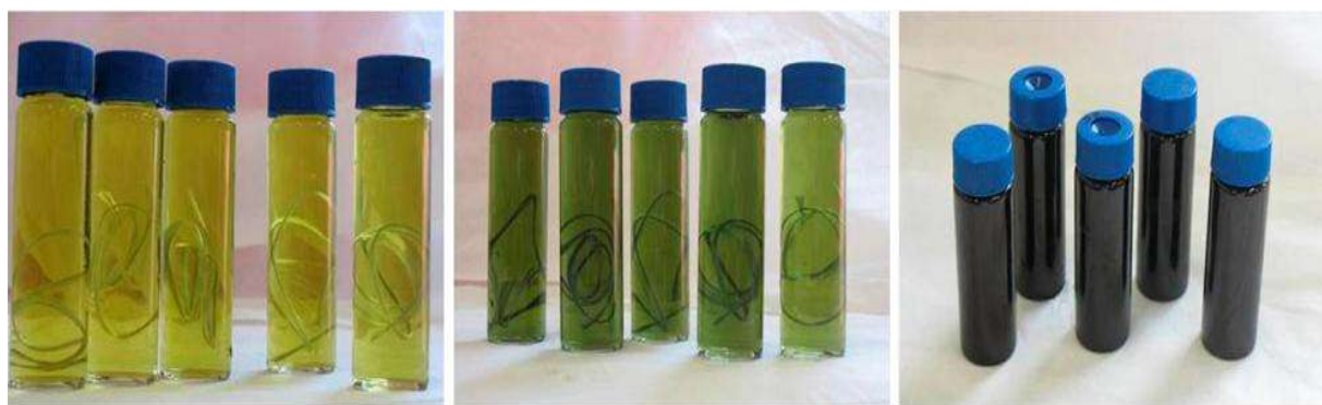
Figure 2. In-situ chemical polymerization by single bath process [59] .
