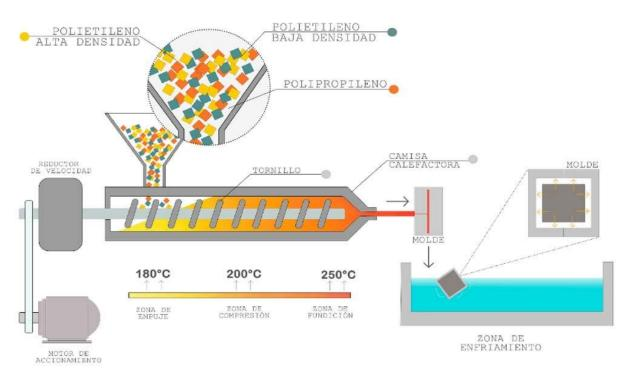
Figure 1. Plastic extrusion-pressure (injection) process.
