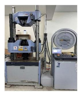
Figure 3. Universal machine UH F500 Kn X.
