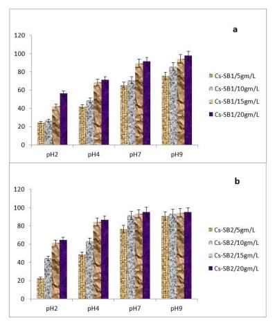
Figure 7. (a) Cs-SB1; (b) Cs-SB2 for *R*% removal of Cu(II) metal ions removal as a function with pH and adsorbent masses
