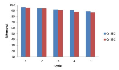
Figure 12. Recyclability of Cs-SB1 and Cs-SB2 adsorbents in removal of Cu(II) ions.
