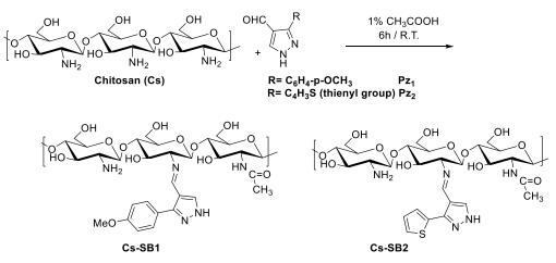
Figure 2. Preparation of the two chitosan-Schiff base derivatives.
