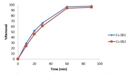
Figure 8. Effect of contact time of Cs-SB1 and Cs-SB2 on metal ions removal %.
