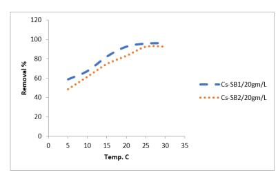
Figure 9. Effect of temperature on metal ions removal % by Cs-SB1 and Cs-SB2.
