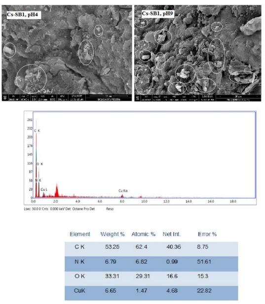
**Figure 10.** SEM image of Cs-SB1/Cu(II) at pH of 4 and 9, its EDX profile and analysis of elemental constitutes in weight %.
