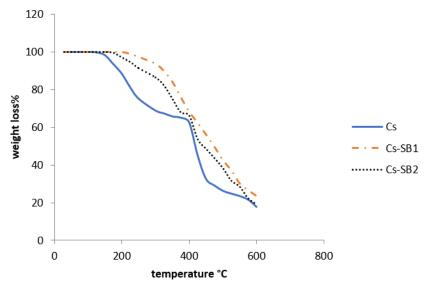
Figure 5. TGA of Cs and its Schiff bases, Cs-SB1 and Cs-SB2.
