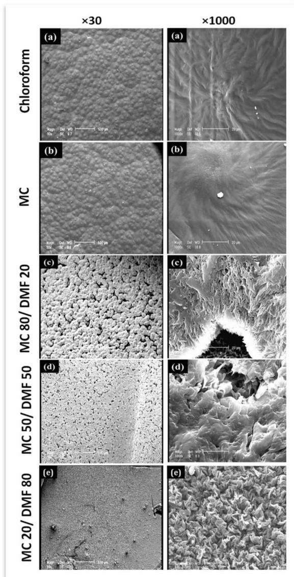
**Figure 2;** SEM micrographs of the prepared films using (a) Chloroform, (b) MC, (c) MC 80/ DMF 20, (d) MC 50/ DMF 50, and (e) MC 20/ DMF 80 solvents at two magnifications ( $\times 30$  and  $\times 1000$ ).
