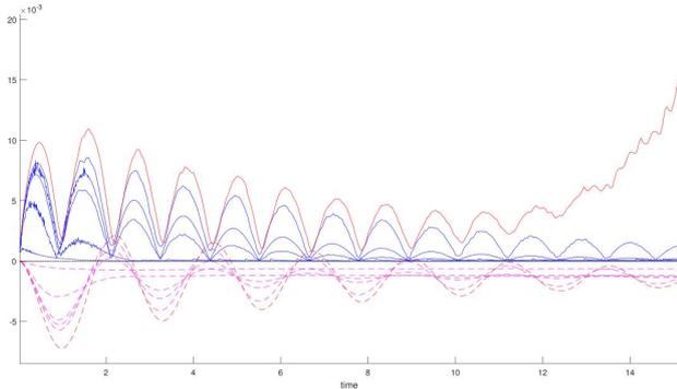
**Figure 3;** Time dependencies of the non-stationarity functional (8) (solid lines) and inlet fluid volume fluxes (dashed lines). The blue solid lines (in ascending order) and magenta dashed lines (in descending order) correspond to Oldroyd-B fluids with  $De=4$ ,  $Re_p=0.1$ , and  $Re_s$  respectively, 0.1, 1, 5, 10, 100. The red (top and bottom) lines are pertinent to the UCM fluid with  $De=4$ ,  $Re=0.1$ .
