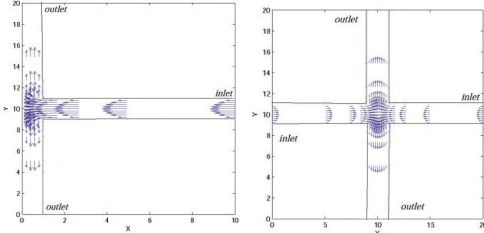
**Figure 1;** Forms of two benchmark flows of viscoelastic fluid: flow against a wall and counterflows within cross slots.
