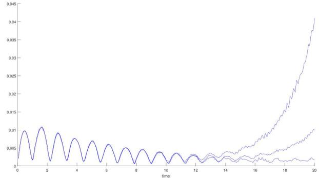
**Figure 4;** Time dependencies of the non-stationarity functional (8) for the UCM fluid flow with  $De=4$ ,  $Re=0.1$ . The calculations are performed on meshes of different fineness: 900, 1296, 1600 nodes in order of the curves increase.
