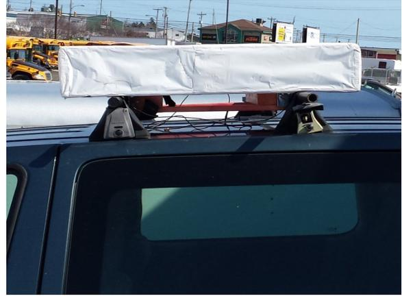
**Figure 10.** The antenna configuration in the ground test.
