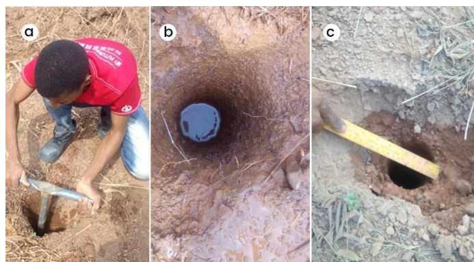
Figure 4. In-situ hydraulic conductivity measurement in the field.
