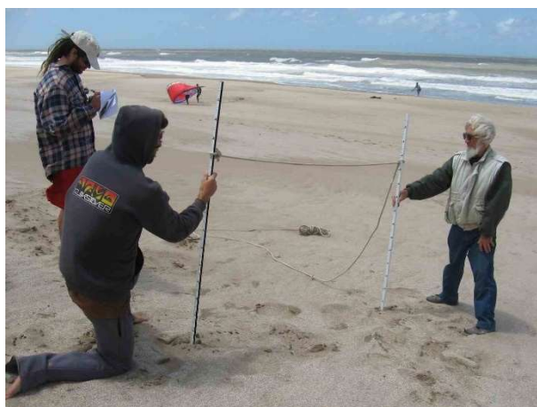
Figure 6. Measurement of beach profiles with the method developed by Bustos [29] .
