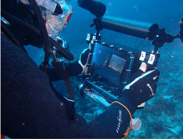
**Figure 1.** Custom underwater video camera developed to acquire images by a diver.
