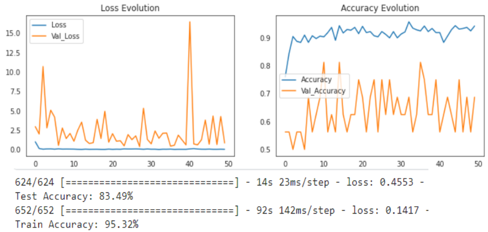
Figure 9. Loss and accuracy values of CNN Model for test and train input.
