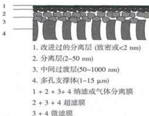
Figure 1. Schematic diagram of the principle of asymmetric composite film
