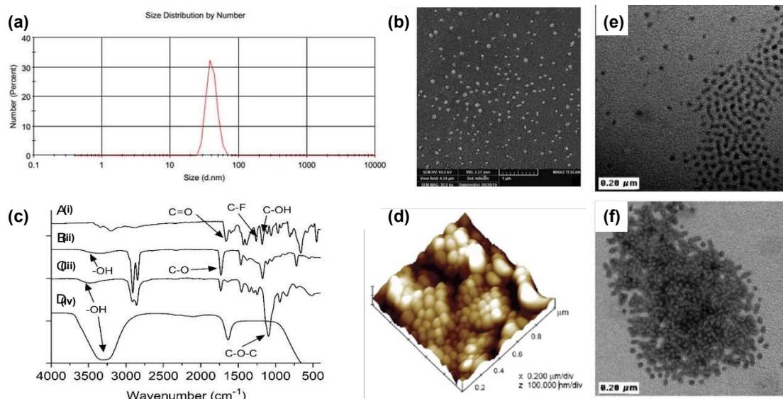
**Figure 5.** (a–b) Characterization of PLGA-PEG-PLGA NPs loaded with 5FU@Chrysin; (c) FTIR spectra of (i) Unprocessed (FPV); (ii) Compritol 888; (iii) Tween 80; and (iv) FPV-SLNs; (d) AFM analysis of PEG-g-PLA PNPs' surface morphology; (e–f) TEM photographs of bare and hydrogenated spherical PS/PBD core-shell NPs, respectively. Reproduced with permission from Mostafavi et al. [13], Khaledi et al. [59], Tulbah and Lee [58], and Wang et al. [60], respectively.
