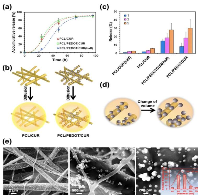
**Figure 12.** CUR release from PCL/CUR and PCL/PEDOT/CUR MFs. **(a,c)** CUR release profiles in PBS-EtOH, and after electrostimulation by applying 1, 3, and 5 consecutive potential pulses, respectively; **(b,d)** Scheme representing the diffusion mechanism for CUR release in the absence/presence of electrostimulation, respectively; **(e)** SEM micrographs of PCL/PEDOT/CUR fibers after electrostimulation. Reproduced with permission from Puiggali-Jou et al. [84].
