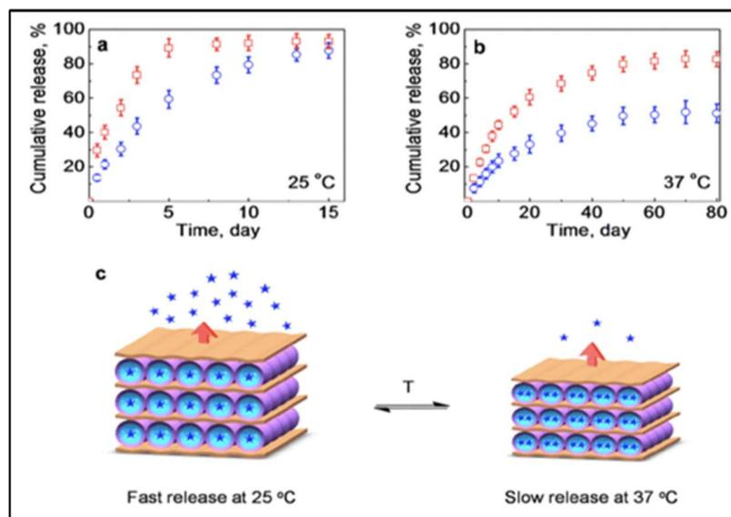
**Figure 8.** Release kinetics of FPV from [SNC-g-PNIPAM-b-PDMAEMA/PMAA]<sub>3</sub> (squares) and [SNC-g-PNIPAM-b-Q100M/PMAA]<sub>3</sub> (circles) films at (a) 25 and (b) 37 °C; (c) Schematic representation of mechanism. Reproduced with permission from Xu et al. [79].
