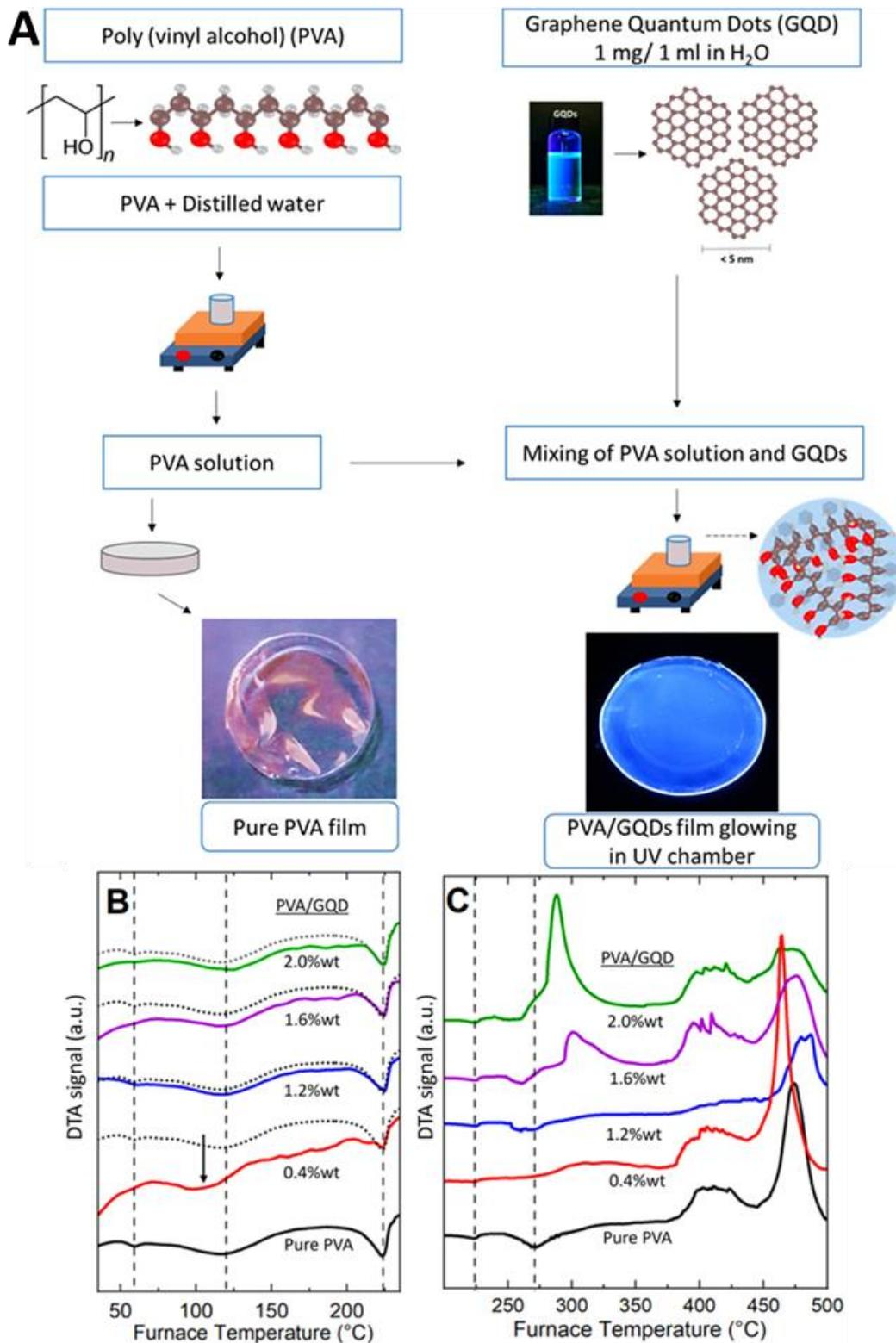
**Figure 6.** (A) Fabrication of pristine PVA and PVA/GQD nanocomposite films; (B,C) differential thermal analysis data of neat PVA and PVA/GQD nanocomposite films, respectively [75]. PVA = poly(vinyl alcohol); PVA/GQD = poly(vinyl alcohol)/graphene quantum dots nanocomposite. Reproduced with permission from MDPI (open access).
