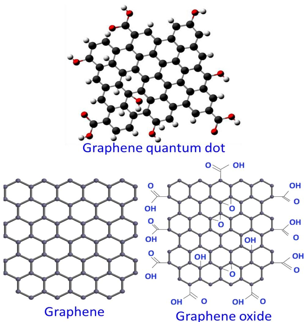
**Figure 2.** Structures of graphene, graphene oxide, and graphene quantum dots.
