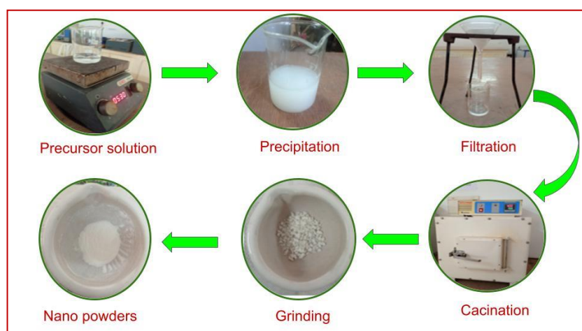
Figure 1. Steps to synthesize zinc oxide nanoparticles.
