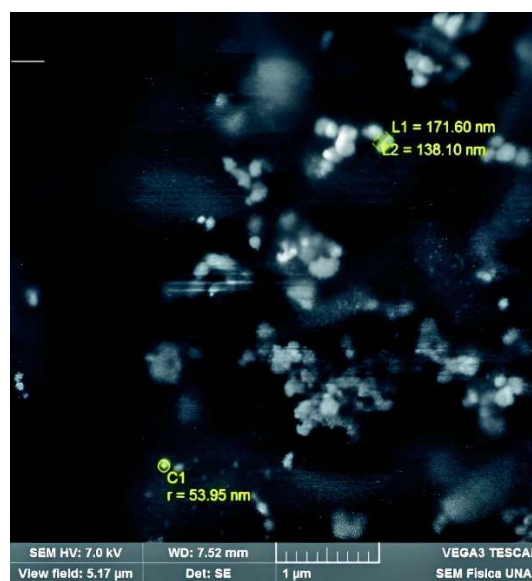
Figure 4. SEM image of the silver nanoparticles obtained with the supernatant of the Chlorella sp. Culture at room temperature and 10% glycerol.
