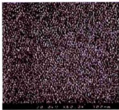
b. Cu 2 O/TiO 2 composite film (Cu 2 O sputtering time is 30s)
