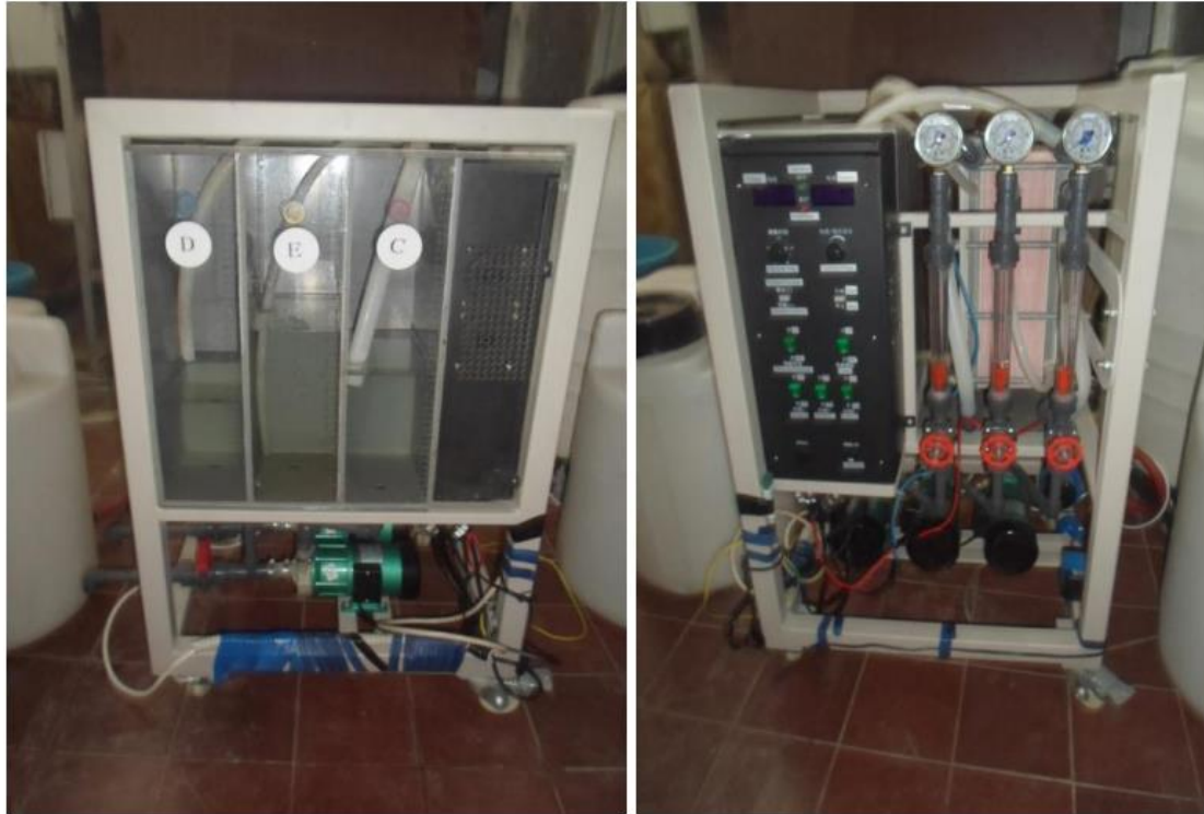
Figure 1. Electro dialysis unit (IONLYZER-40-2040, IONTECH Co., China).
