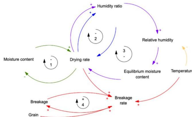
**Figure 1.** Causal diagram of the system dynamics breakage model<sup>[21]</sup>.
