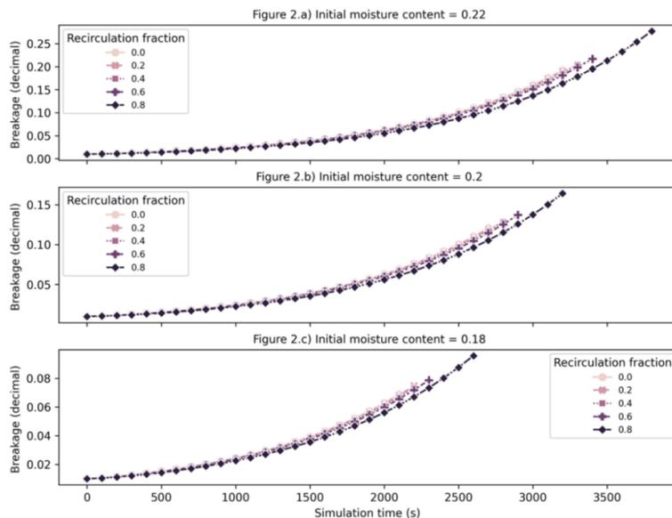
**Figure 2.** Effect of initial moisture content under breakage dynamics.
