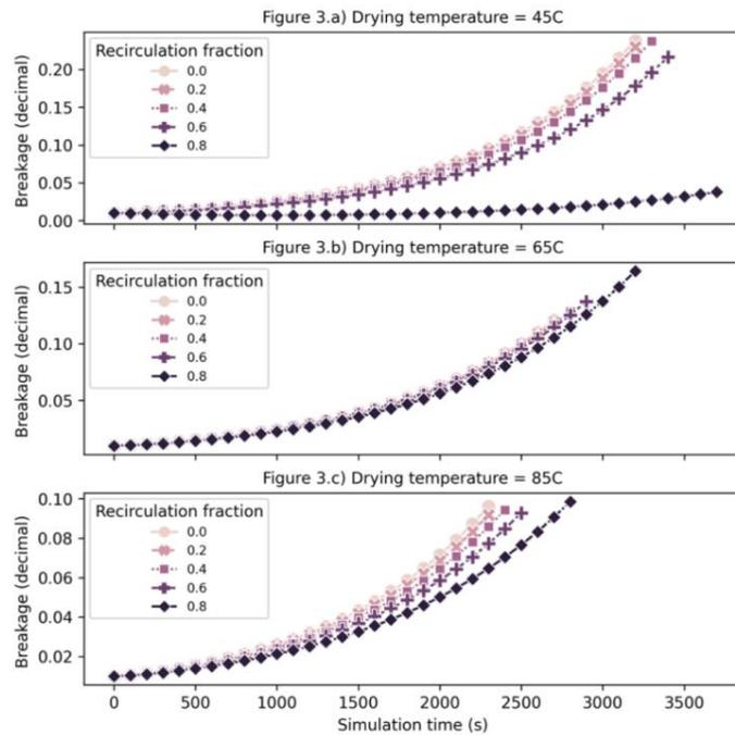
**Figure 3.** Effect of drying temperature on breakage dynamics.
