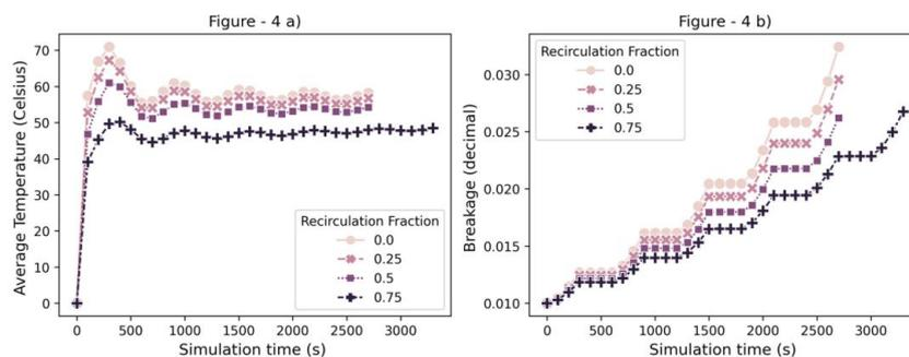
**Figure 4.** Time profiles for the intermittent drying experiment: (a) Average drying temperature temporal profile; (b) Product breakage temporal profile.
