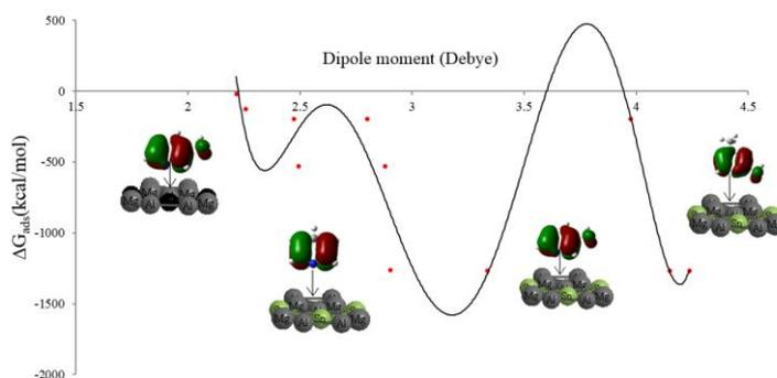
**Figure 3.** The Gibbs free energy for adsorption of pyridine and its derivatives as corrosion inhibitors on the aluminum nanoalloys consisting of Al-Mg-Si, Al-Mg-Ge and Al-Mg-Sn versus dipole moment (Debye).
