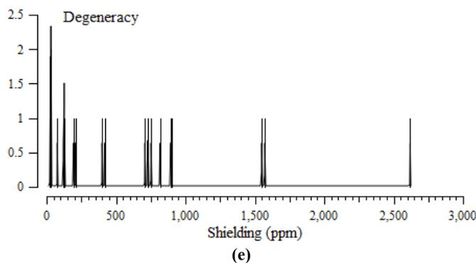
**Figure 1.** NMR spectroscopy for (a) pyridine  $\rightarrow$  Al-Mg-X; (b) 2-picoline  $\rightarrow$  Al-Mg-X; (c) 3-picoline  $\rightarrow$  Al-Mg-X; (d) 4-picoline  $\rightarrow$  Al-Mg-X; and (e) 2,4-lutidine  $\rightarrow$  Al-Mg-X, by showing the active nitrogen atom in heterocyclic compounds becoming close to the nanosurface ( $X = \text{Si, Ge, Sn}$ ).
