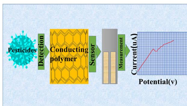
**Figure 8.** Conducting polymer/noble metal nanoparticle nanocomposite-based electrochemical sensor.
