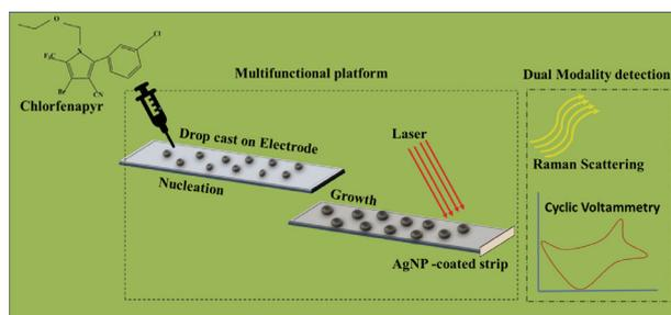
**Figure 6.** Diagrammatic illustration based on binary detection of chlorfenapyr through EC and SERS on test strips coated with AgNP via electrodeposition preparation.
