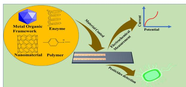
**Figure 4.** The schematic diagram for MOF/nanoparticles/organic/inorganic molecule for working electrode mechanism for pest detection sensor.
