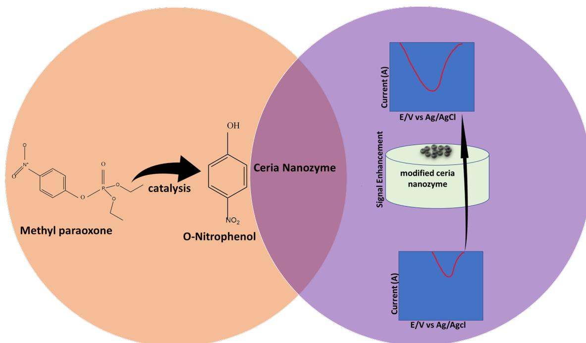
**Figure 9.** Schematically depiction of the electrochemical approach for detecting methyl-paraoxons via bifunctional CeO<sub>2</sub> nanozyme.
