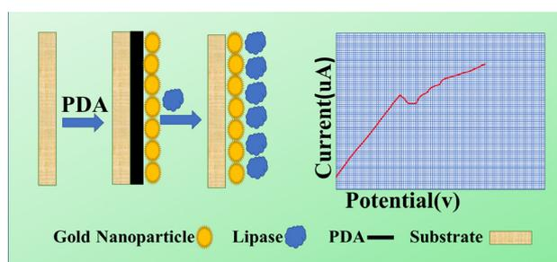
**Figure 5.** Simplified representation for preparation of AuNP/PDA active platform for pesticide selective recognition.
