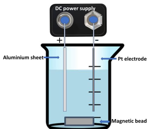
**Figure 10.** Electrochemical setup for aluminium anodic oxidation.
