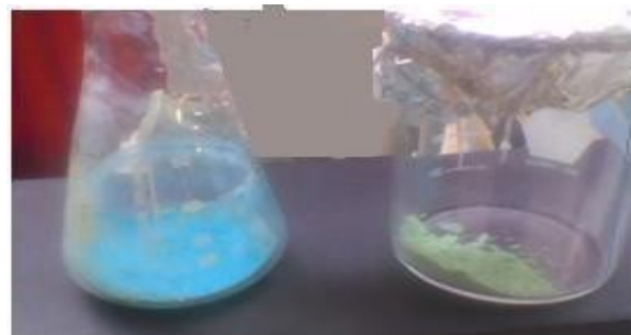
Figure 3. Erlenmeyer flask with the reagent \text{Cu}_3(\text{PO}_4)_2 \cdot 3\text{H}_2\text{O} . Beaker with the product \text{Cu}_2(\text{OH})\text{PO}_4 .
