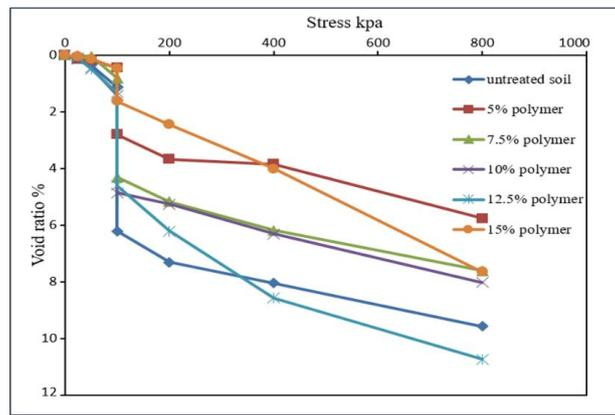
Figure 4. Show the collapsibility test results for soil treated by xanthan gum.
