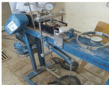
**Figure 2.** Direct shear box test.
