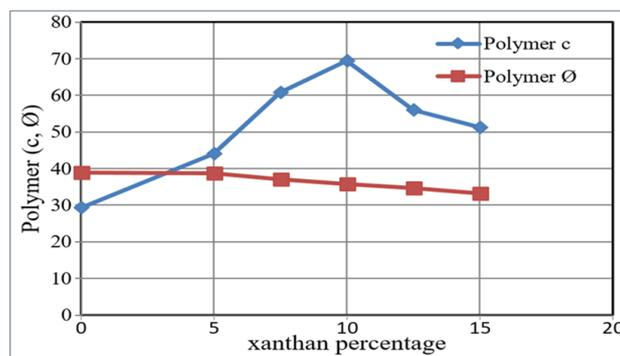
Figure 6. Relationship between the collapse potential and xanthan gum content.
