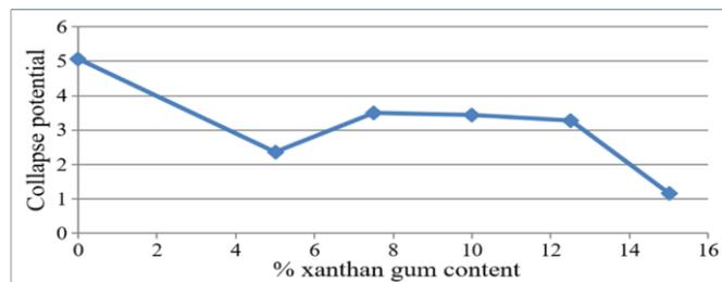
Figure 5. Relationship between the collapse potential and xanthan gum content.
