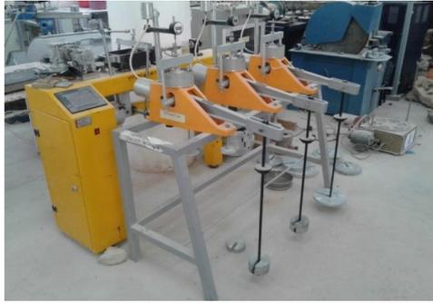
**Figure 3.** Oedometer test.
