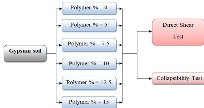
**Figure 1.** The process flow of the test.
