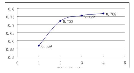
Figure 2. Relationship between microwave frequency and absorbance of gardenia polysaccharide solution
