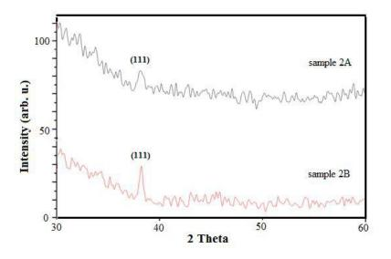
Figure 5. XRD analyze sample2A (up) and 2B (down).
