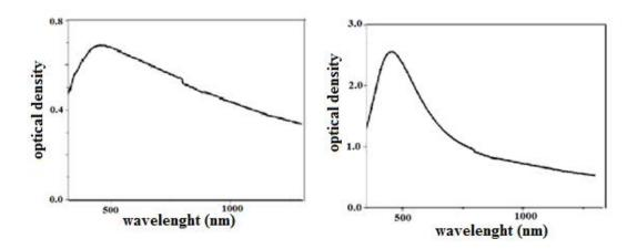
Figure 4. Optical density of sample 2A (left) and 2B (right).
